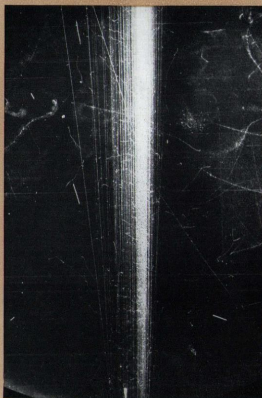
FIGURE 9 - Tracks in a diffusion cloud chamber irradiated by 150 MeV protons from the Harwell synchrocyclotron.
