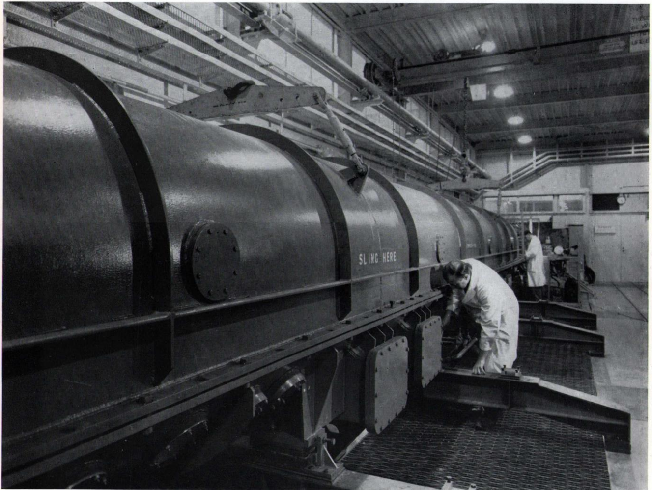
Looking along the outer vacuum envelope of the proton linear accelerator. The 50 MeV accelerating tube, in three sections, is more than one hundred feet long and over this length, axial alignment is accurate to 0.02 inches. Particle accelerators like this are essential tools for the nuclear physicist. His studies of the structure of the nucleus depend upon experiments on the interactions between nuclei and elementary particles at all energies; these machines provide the required particles.
