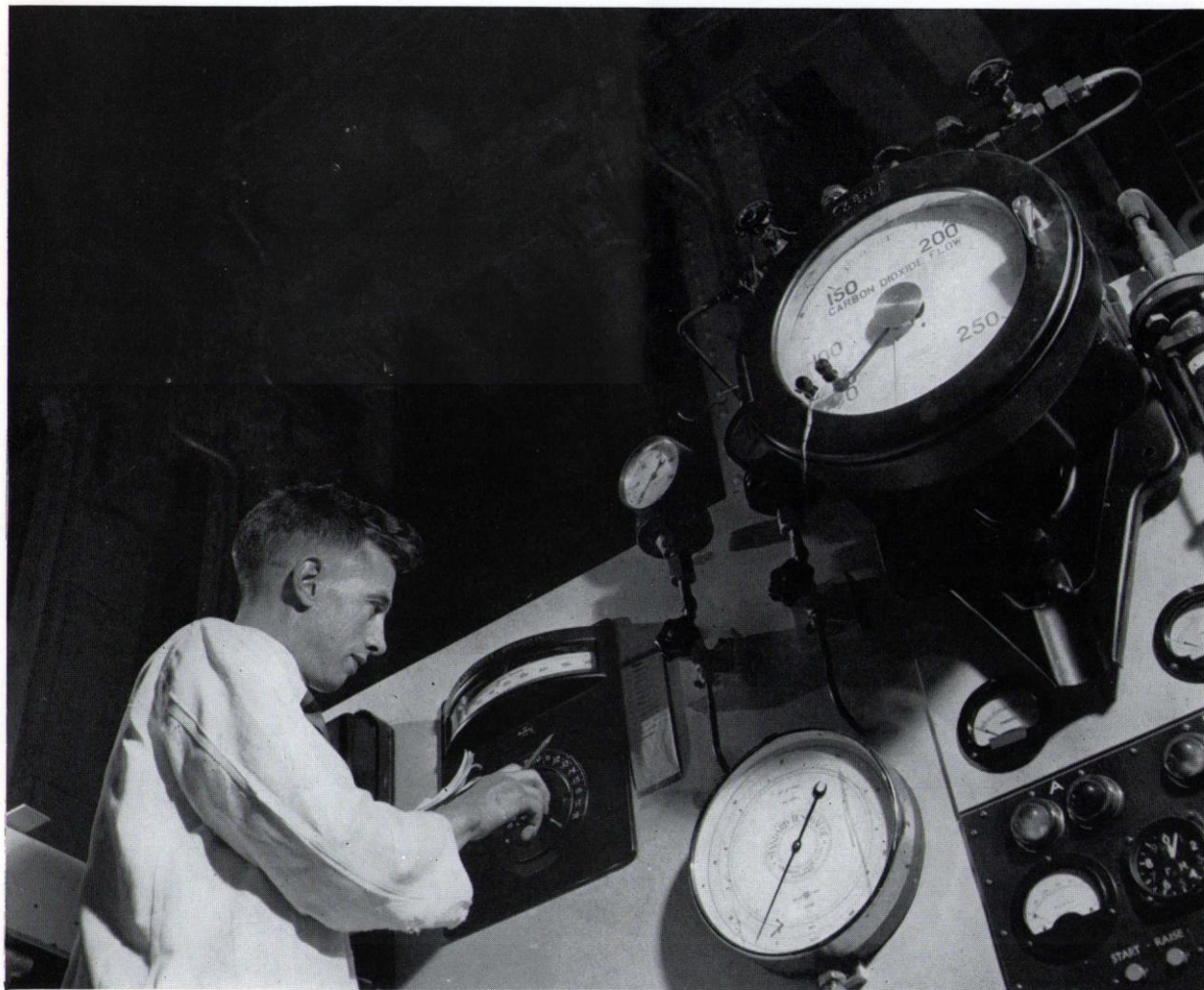
Radiation chemistry on the engineering scale — control panel of a 'loop' in Bepo for measuring the rate at which carbon dioxide reacts with graphite under power-reactor conditions. A loop is a closed circuit through the pile core; this one contains a graphite channel loaded with fuel elements.
