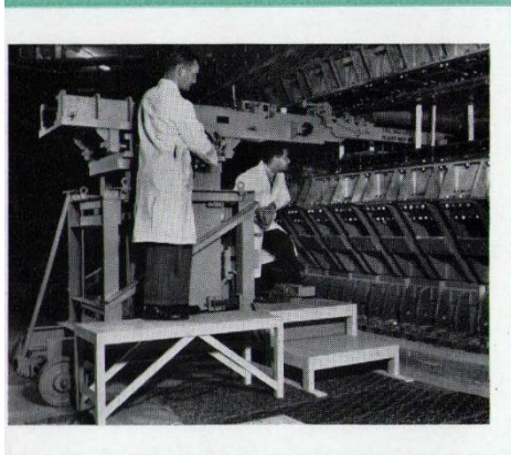
◀ Assembling the pole pieces in the throat of the magnet. Each of the 672 pole pieces had to be positioned within a few thousandths of an inch in relation to the magnet sectors.
