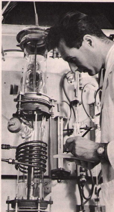
An experiment at tracer level to study the release of particulates and gaseous fission products from hot uranium in a stream of coolant gas
