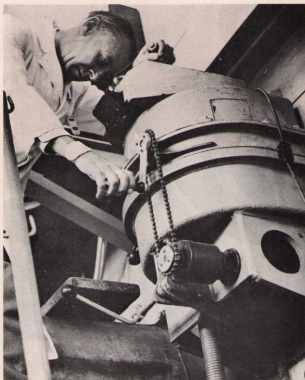
Isotope production: loading cans of material for irradiation in BEPO
