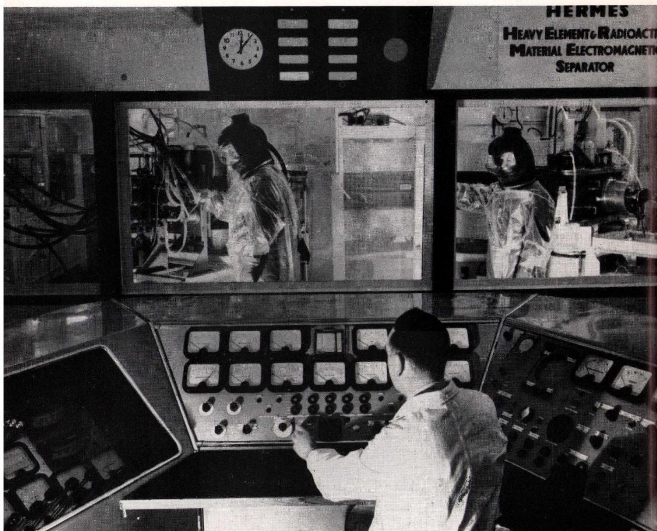
HERMES (Heavy Element Radioactive Material Electromagnetic Separator) in operation. Looking from the control desk into the active room, the radioactive source is shown on the left and the collector on the right: Engineering Division, Harwell
