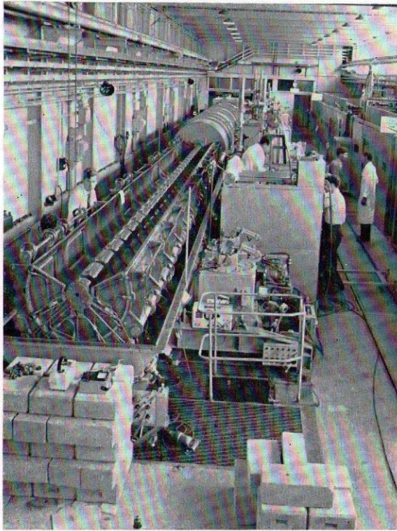
Tank 3 of the P.L.A. showing the drift tubes; the vacuum cover and the liner lid are removed.
