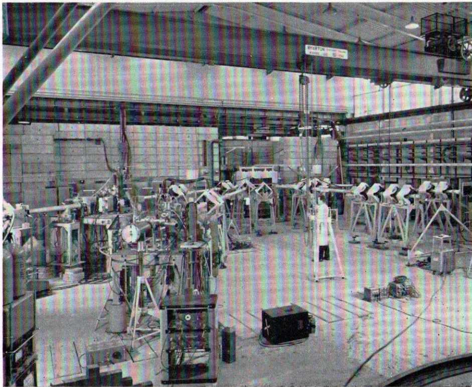
Part of the new P.L.A. Experimental Area showing the alternative beam pipes radiating from the bending magnet.
