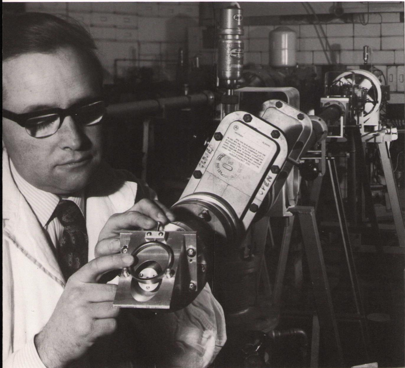
A valve seating being positioned in the irradiation jig
