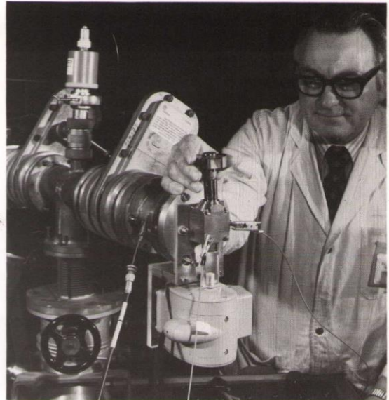
An injection rotor being positioned in the irradiation jig
