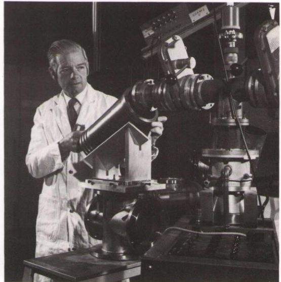
A cylinder liner being positioned in the irradiation jig
