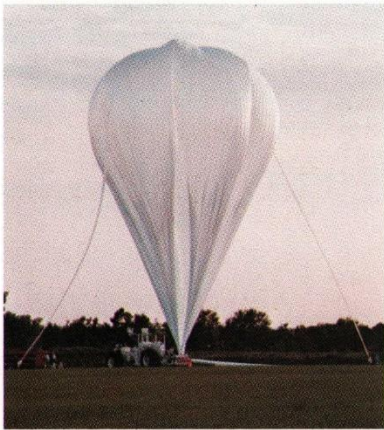
Inflating a million cubic foot balloon which will support the stabilised balloon platform.
