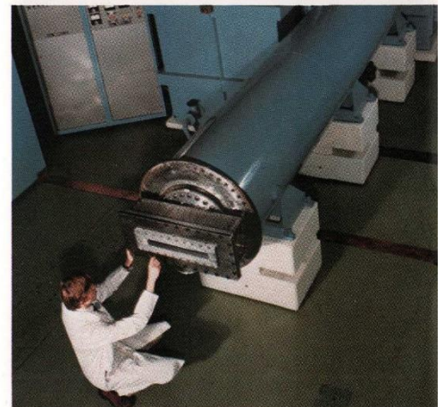
"ELF" — a high current electron beam generator for gas laser research.
