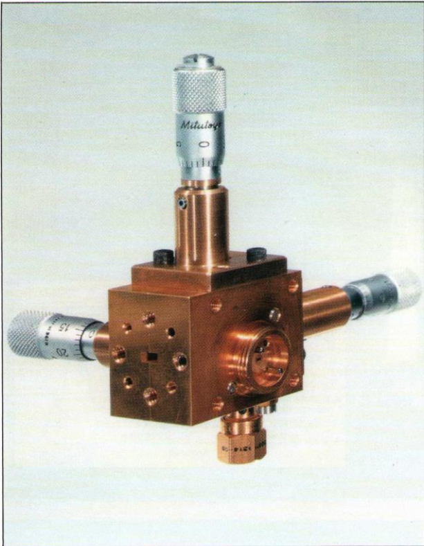
Above: The 345 GHz receiver made at Radiosterrenwacht Dwingeloo in the Netherlands.
