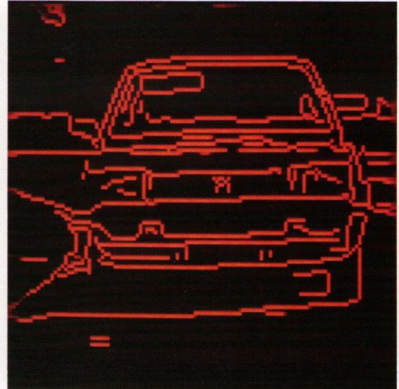
2.6 Image of car shown in Fig 2.5 after processing to label edges using probabilistic relaxation. (87RC3494)
