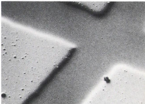
Figure 7: Patterned polycrystalline film of high T_c YBCO. These films were deposited by excimer laser ablation from bulk material on to heated substrates.
