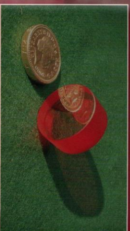
24 mm diameter Ti:Sapphire crystal
