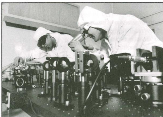
Goncalo Figueira, University of Lisbon, and Colin Danson, RAL, align one of the amplifiers on the new laser shortly before completion
