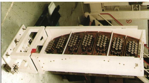
A view of one half of the new detector array prior to installation and assembly of the shielding around the detectors
