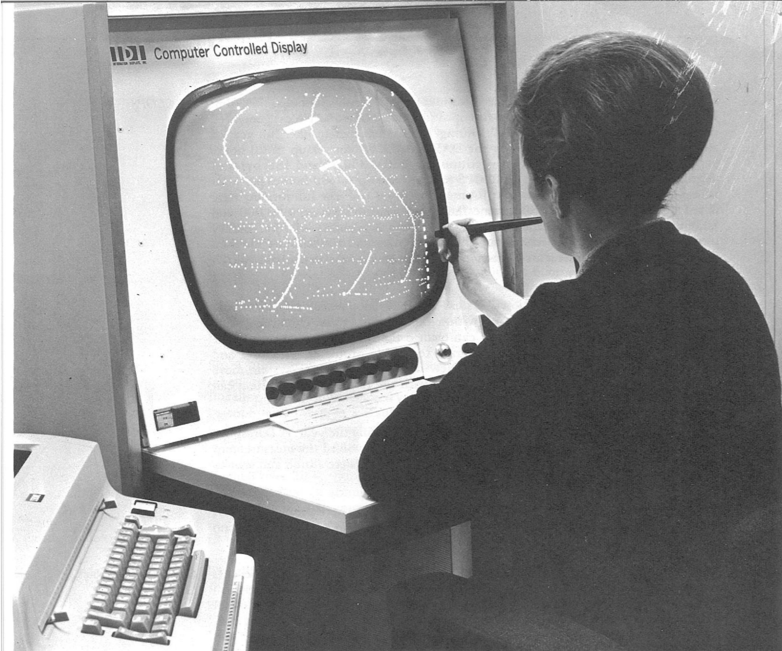
Figure 95. Selected events shown on a computer controlled display. By means of a light-pen the operator controls the selection and accurate measurement of bubble chamber events.
