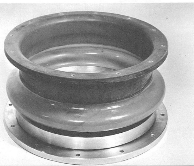
Figure 105. Model bellows made from fibre-glass cloth bonded with epoxy resin.
