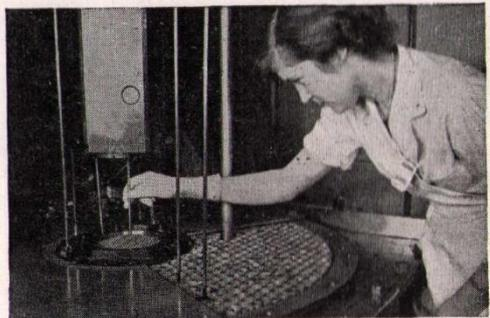
**5. ZEPHYR** (Harwell). Zero Energy Fast Fission Reactor. The first "fast" research reactor to be built in Britain; it began working in 1954. Its core fuelled with plutonium, is a cylinder 6 ins. dia. by 6 ins. long. Fast reactors such as Zephyr can produce as a by-product more fuel than they burn.
