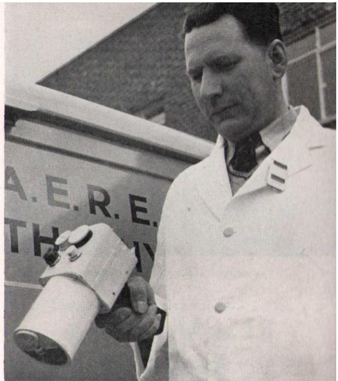
Health Protection at Harwell—a portable geiger counter used for checking radioactivity.
