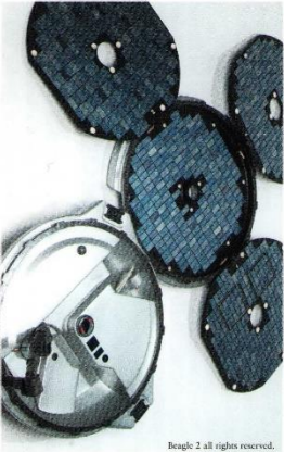
The Beagle 2 lander showing its solar panels outspread and its instrument arm being deployed.
