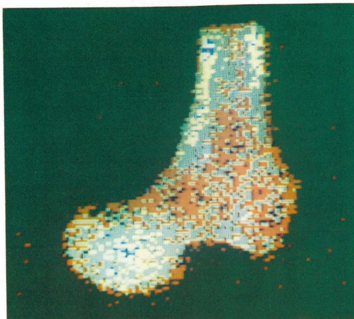
Computer display of bone density based on the transmission of X-rays through part of a human femur, each colour is set to represent a given density range.
