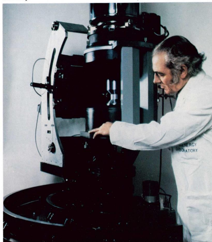
Left. Dilution refrigerator for the ^{149}\text{Sm} polarising filter under test at the Rutherford Laboratory.
