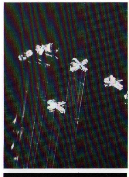
Figure 3: Fine microscopic cell wall creases in a radial longitudinal section of Sitka spruce after 500 cycles of load at 75% of the ultimate flexural strength.
