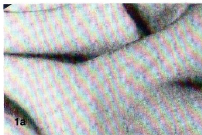
Figure 1: (a) Textile fabric showing multiple three-fold buckling.
