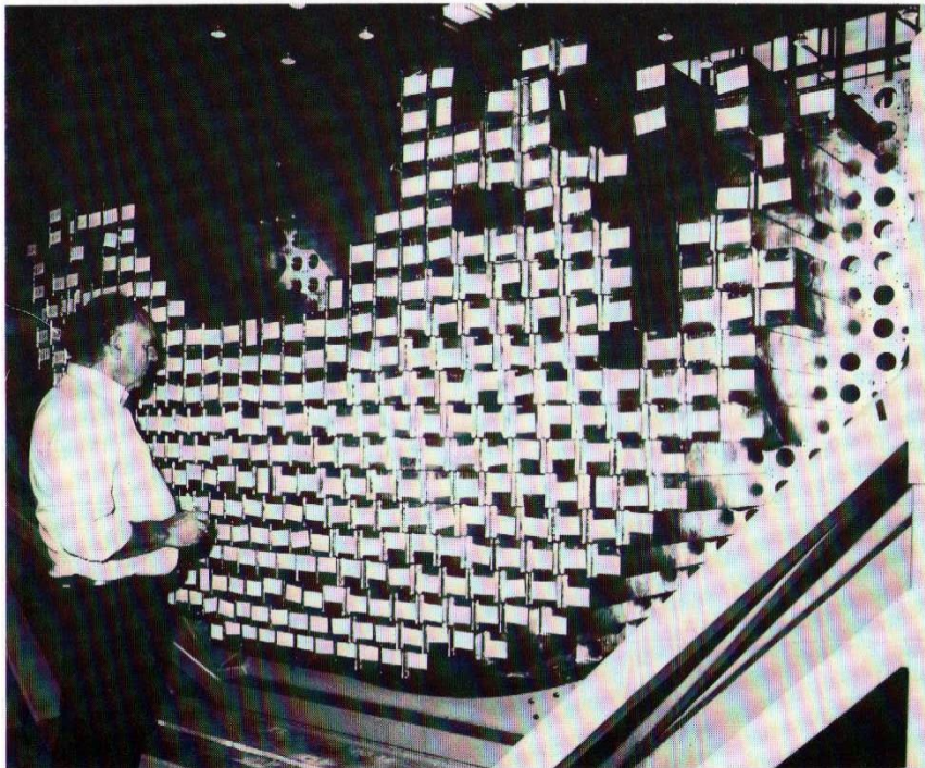
The first calorimeter nearing completion. The lead glass blocks, weighing 17 kg, are supported in brass cans only 0.5 mm thick. (Photo CERN)
