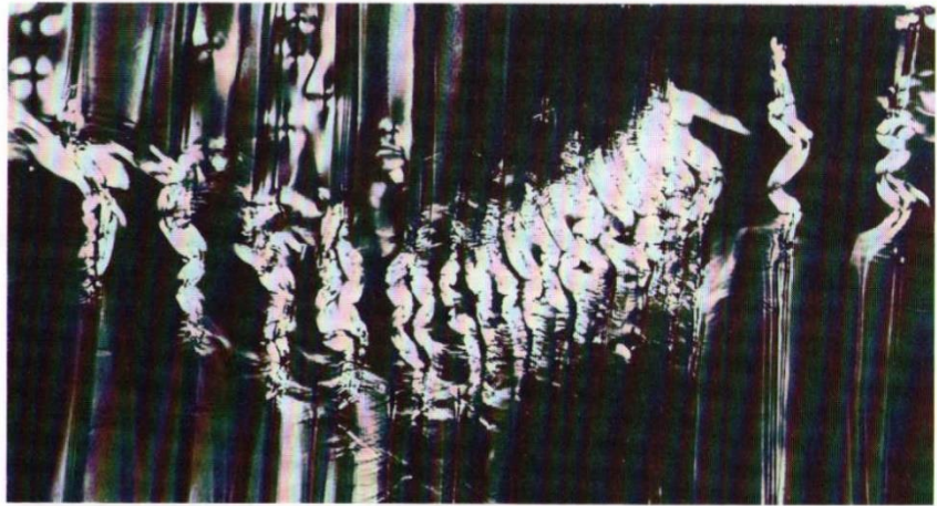
Figure 4: Extensive cell wall rupture after 10^5 cycles. Crossed circles are cell wall pits viewed under polarised light.
