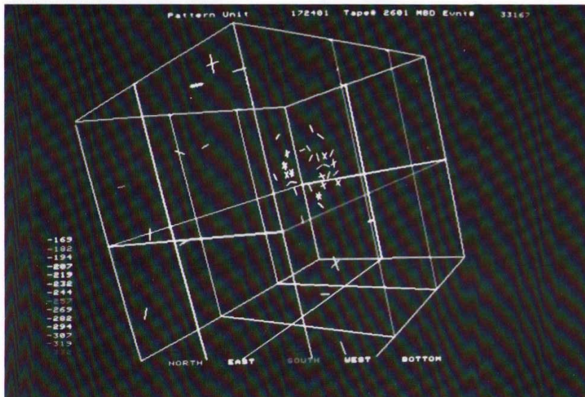
Supernova neutrino event in the IMB detector. The straight lines show the detector walls. The crosses marking the hit phototubes show clearly the intersection of the Cerenkov light core from the positron, with the detector walls.
