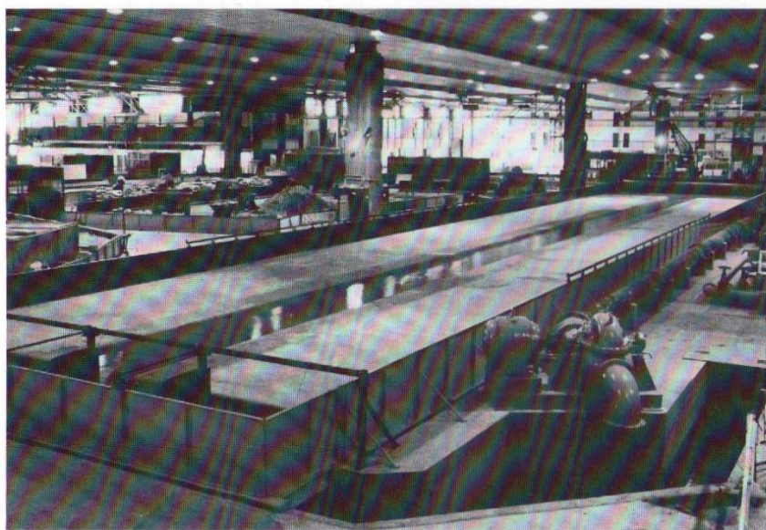
View of the SERC Flood Channel Facility at Hydraulics Research Ltd. The tank is 56 metres long, 10 metres wide and 1 metre deep with a base moulded in cement mortar to the required geometry.
