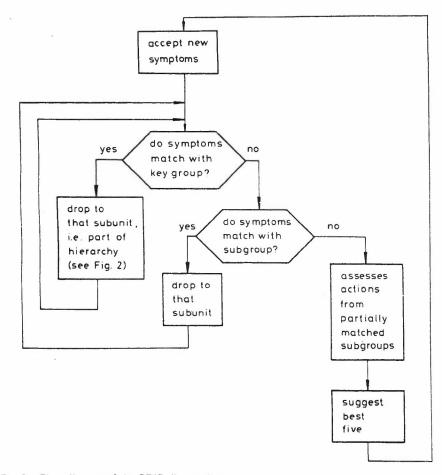
Fig. 3 Flow diagram of the CRIB diagnostic process
