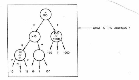
Fig. 11 A single complex test as a set of primitive tests
