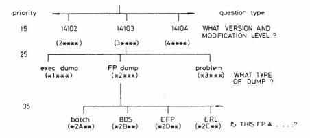
Fig. 5 Part of the VME/K faults database structure
