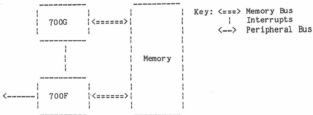
The three sites are linked via the peripheral bus of each of the Argus 700Fs to a fast inter-site bus into which is also connected an Interdata 70 computer. This Interdata 70 which serves as a peripheral and maintenance processor for the entire system runs existing software and is linked through a high speed local network to standard peripherals and the Department's file processor. The interconnection of the sites is shown below.
