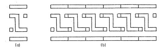
Fig. 3.1.2 Interconnections using closed shapes
