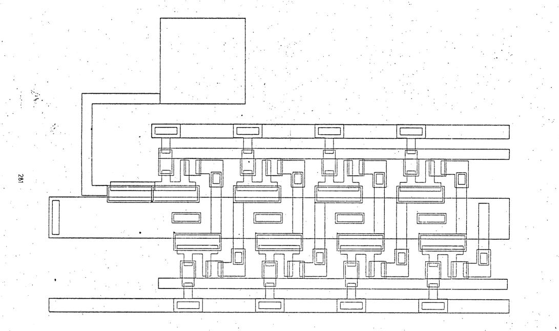
Fig 8.2 Layout of small circuit with grouped and repeated shapes
