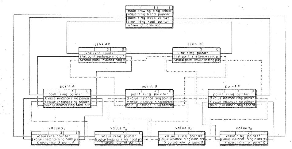
FIGURE 4.15 original myriad data structure for two line segments
