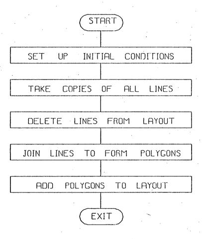
FIG 7 7 1 SIMPLIFIED FLOW DIAGRAM OF GAEL6A
