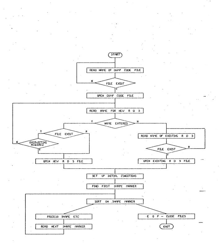
FIG 7 4 1 SIMPLIFIED FLOW DIAGRAM OF CAELSA
