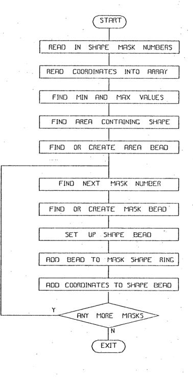
FIG 7 4 2 FLOW DIAGRAM OF RECTANCLE PROCESS
