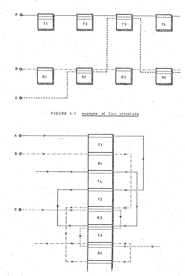
FIGURE 4.2 Layout of structure in memory
