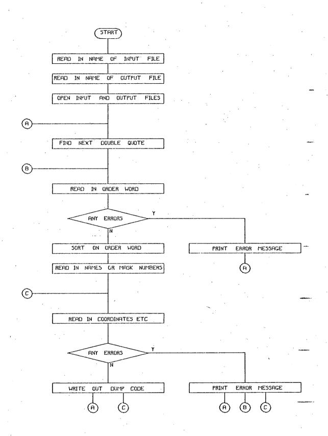
FIG 7 3 1 SIMPLIFIED FLOW DIAGRAM FOR GREL2A
