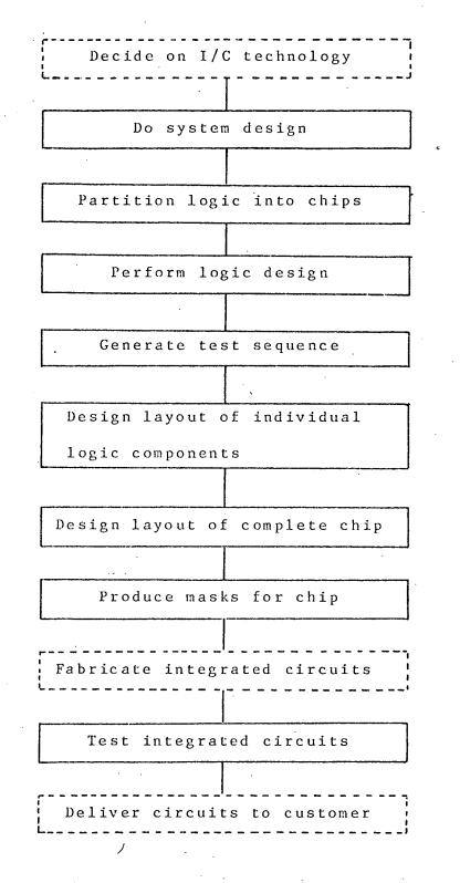
Fig. 1.1 Flow diagram for integrated circuit manufacture
