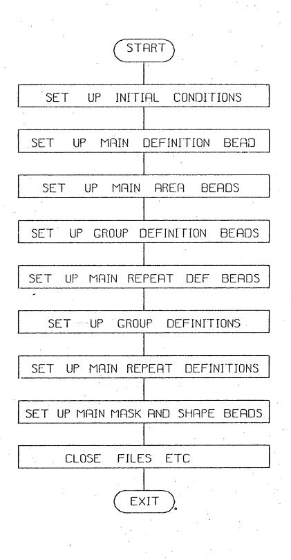
FIG 7 9 1 SIMPLIFIED FLOW DIAGRAM OF GAELBA ----
