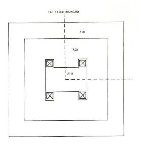
FIGURE 5 - Boundary integral method model using symmetry - the far field boundary is infinity
