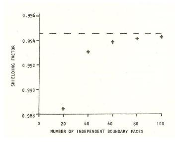
FIGURE 7 - Shielding factor of a hollow ferromagnetic cylinder – dimensions as figure 6, permeability 1000 - as a function of the number of independent boundary faces.
