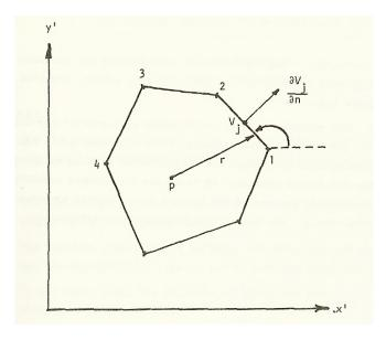
FIGURE 12 - Global coordinate system A boundary surface subdivided into elements
