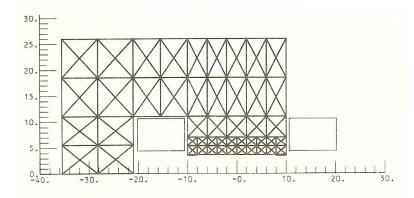
FIGURE 8 - GFUN Model of a two-dimensional C-magnet
