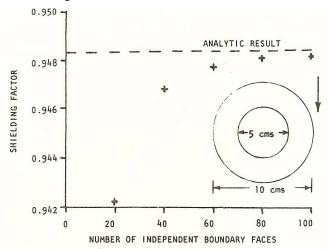
FIGURE 6 - Shielding factor of hollow ferromagnetic cylinder – Inside Radius 5 cm. Outside radius 10 cm. permeability 100 - as a function of the number of independent boundary faces in the model.
