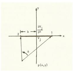
FIGURE 13 - Local coordinate system of an element
