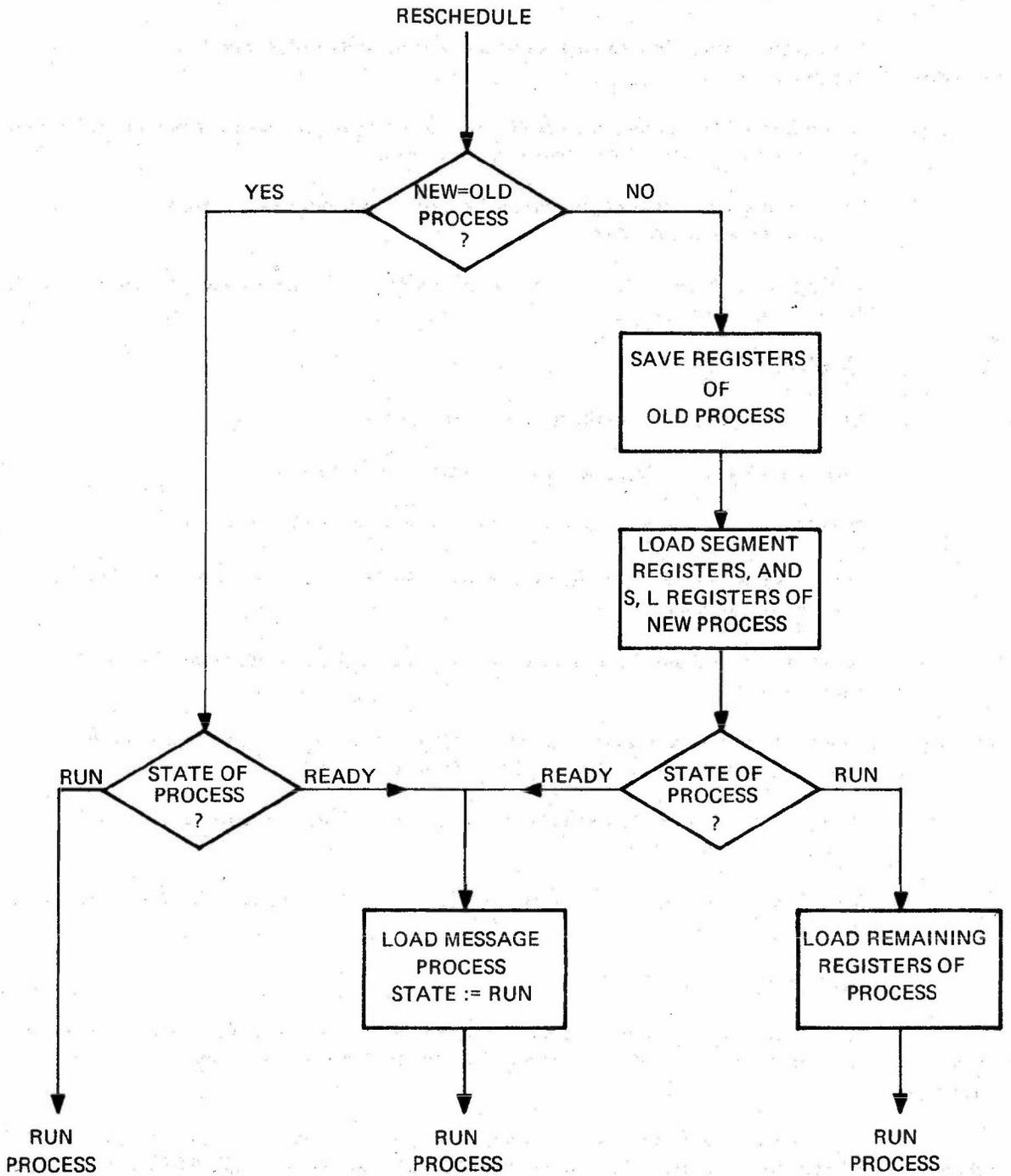
Figure 18: PROCESS CHANGE MECHANISM
