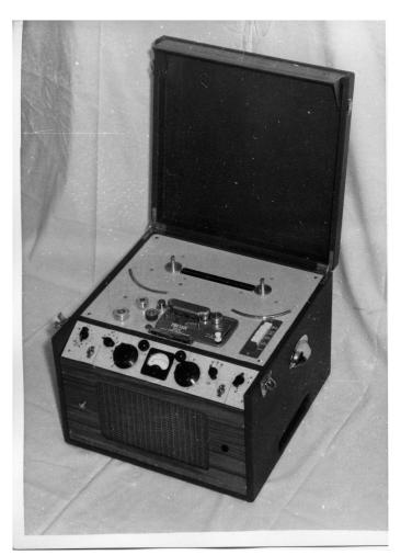
Home built tape recorder, based on a Truvox deck.
