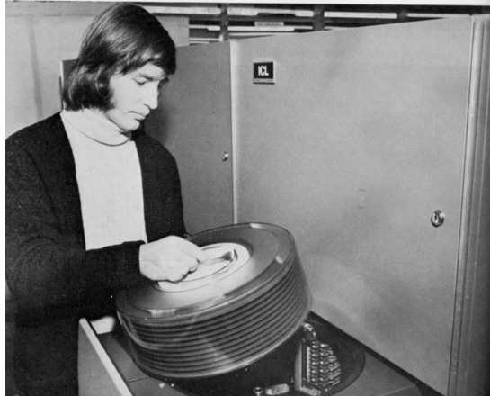
Swappable “hard disk pack”. Not very big (< 500Mb?) and prone to crashing!
