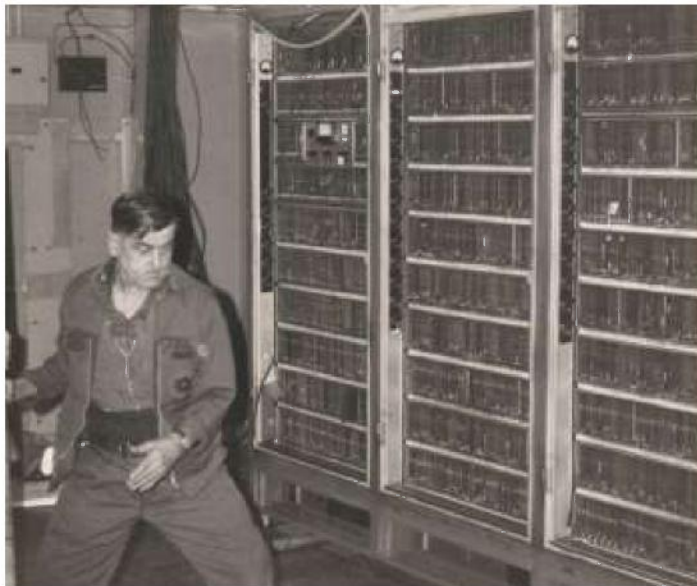
One of the bays showing the thousands of printed circuit cards which constituted a large part of the computer.
