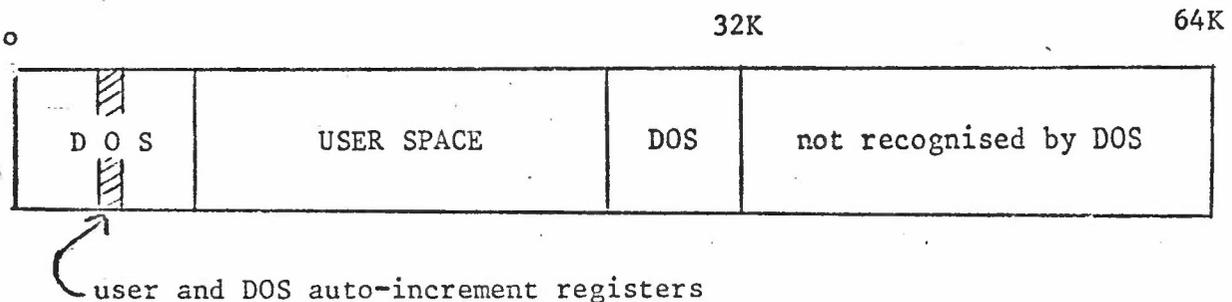
Figure 4.1 DOS CORE LAYOUT
