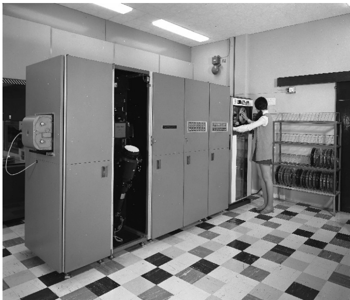
Tape loading the SC4020, with image tube visible
