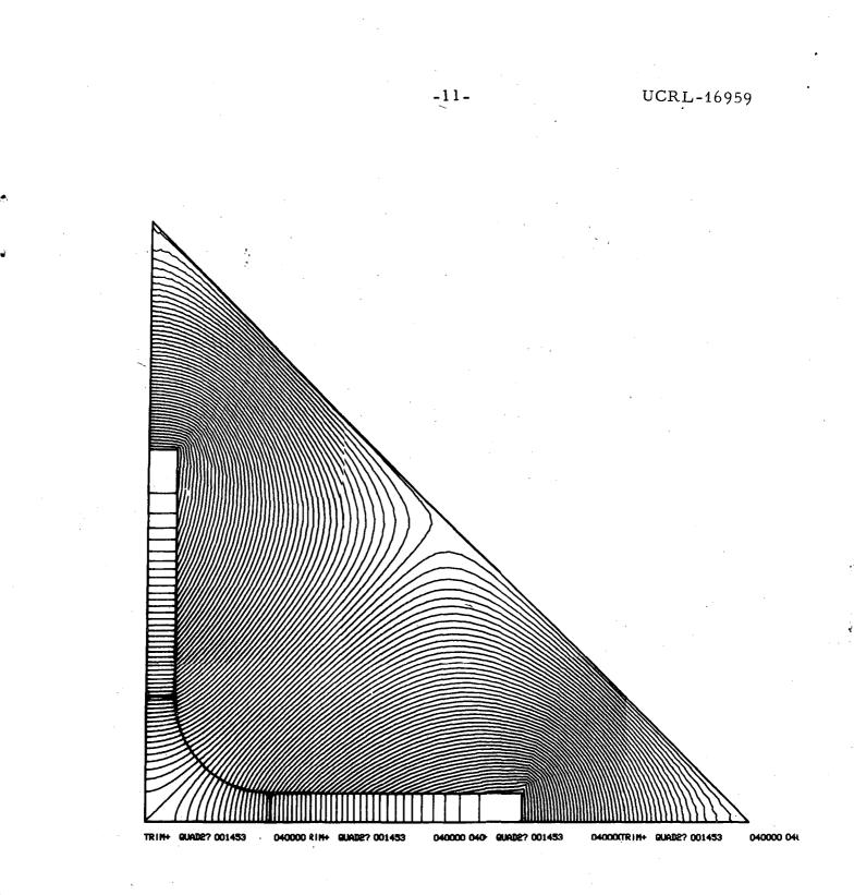
Fig. 7(c) CRT plot of flux distribution for the quadrupole magnet shown in Fig. 7.
