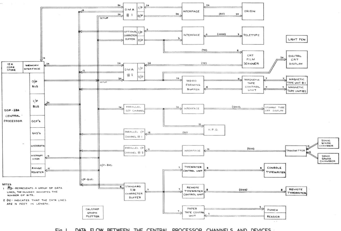
DATA FLOW BETWEEN THE CENTRAL PROCESSOR CHANNELS AND DEVICES Fig. I
