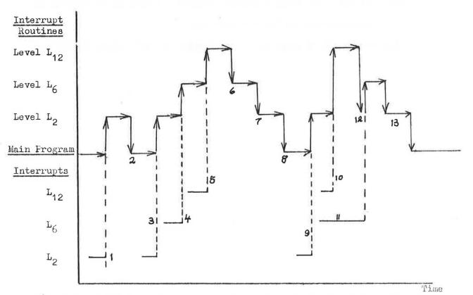
1) A level 2 interrupt occurs causing a jump to the level 2 routine.
