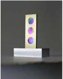
Formvar (a type of plastic) foils on a three-target holder. Even in the early days, thin foil targets were in demand although not in the quantities required for microspheres. (23199)
