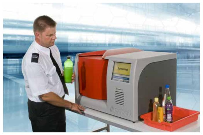
Work on SORS techniques has led to the development of the Insight100 machine, a bottled liquid screener for use in airports. This was developed and marketed by an STFC spin-out company Cobalt Light Systems Ltd. There are about 400 operational units in 70 airports across Europe and Asia; Heathrow alone has over 80. It is hoped that this technology will allow the relaxation of airline restrictions on bringing liquids on board aircraft.
