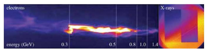
Raw images of characteristic electron spectra and the corresponding X-ray beams.
