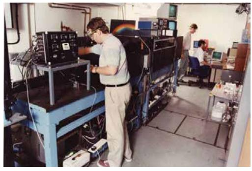
Tony Parker setting up a copper-vapour laser in the Time-Resolved Resonance Raman (TR<sup>3</sup>) facility, 1992. (92RC3455)
