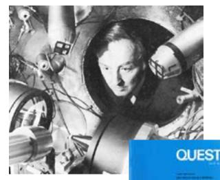
Alan Gibson, head of the Laser Facility, looks inside the laser target vessel showing small stem supporting micro balloon target sphere. (Keystone Press)
