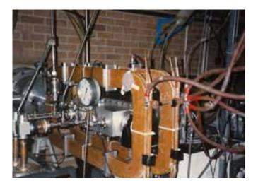
Sprite used an e-beam pumped KrF pre-amplifier laser system named Goblin. This was behind a brick wall in a rather inaccessible part of the laboratory so this is the only photo we can find.
