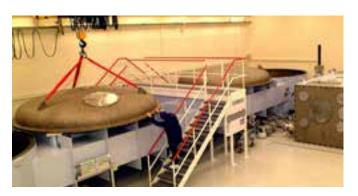
Three-section compression chamber. The "shipping container" target chamber (right) is made of 125 mm thick mild steel, is 5m x 3m x 2m in size, and weighs 60 tons. It is now surrounded by 100 tons of lead (about half of which was supplied by the ISIS facility), 50 tons of concrete, and 20mm thick aluminium plates, 2002. (02EC1630)
