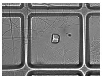
Laser tweezers loading micron-sized protein crystals on micro-meshes covered with a spider's-web of electro-spun fibres, 2013. This work was done in collaboration with Diamond Light Source.
