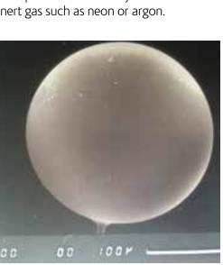
Glass shell micro-target glued to carbon fibre.
