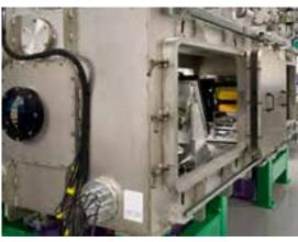
South compressor chamber installed, 2007. One of the gold-coated gratings used for pulse compression can be seen at the far end of the chamber. (07EC3604)
