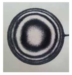
To be useable in experiments, the targets had to be absolutely spherical, have a smooth surface finish and uniform wall thickness. Quality was verified by examining the fringe pattern on an interference microscope, such as the one seen here.
