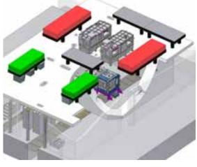
3D CAD visualisation of Gemini Laser Area 3 and Target Area 3, viewed from the north east corner. The green blocks are the two Quantel pump lasers; the red blocks are the north and south amplifers with two compression chambers between. The target chamber for TA3 (purple legs) is just seen on the floor below.
