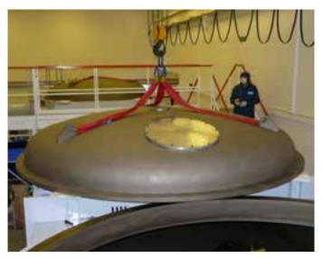
Each day, the two 4.5 metric tonne compressor lids were craned off before work could start. This operation alone took an hour each time, but the delay was mostly due to housework as you cannot open up a clean vacuum vessel unless you are confident that the area outside is as dust-free as possible.
