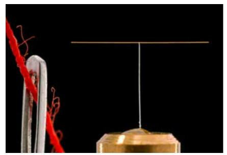
Thin wire target. The top wire is made from gold and is 20 microns in diameter (about a quarter the width of a human hair). (A micron is 10<sup>-6</sup>, or one millionth of a metre.) One end of the gold wire has been polished to sub-micron smoothness, 2005. (05EC4316A)
