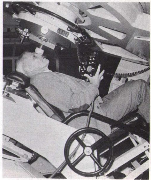
Astronomer-Royal Sir Richard Woolley operating the telescope by means of a remote control box from a specially designed seat at the Cassegrain focus.
