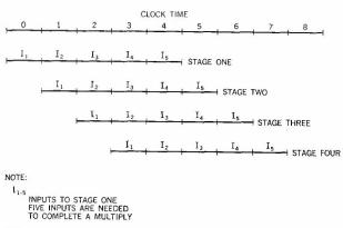
Figure 15 Timing diagram for abstracted iterative hardware.
