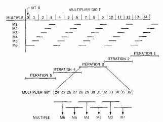
Figure 9 Iterations and multiple generation for multiply.
