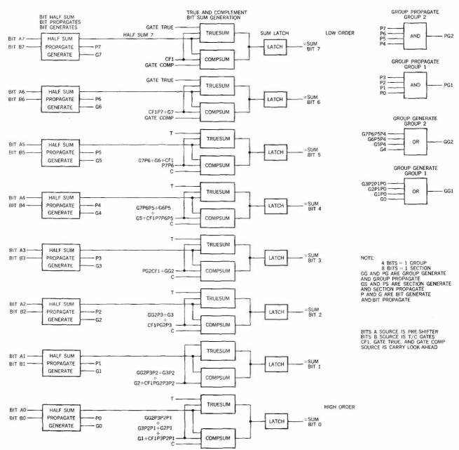
Figure 6 Fraction adder, section 1 (high-order).
