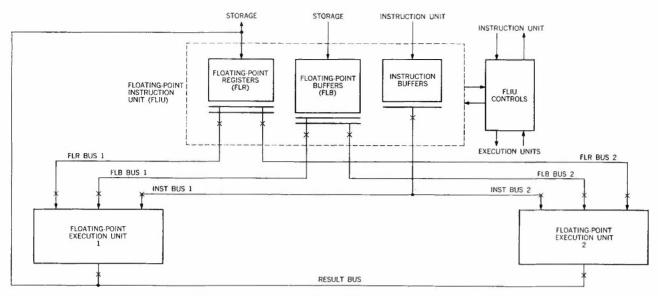
Figure 1 Floating-point execution unit capable of concurrent execution.
