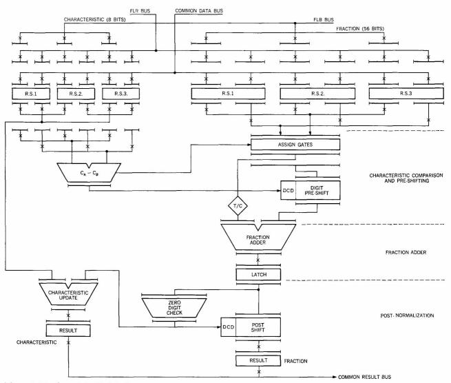
Figure 3 Floating-point add data flow.
