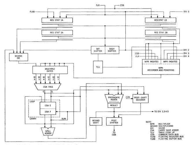
Figure 11 Floating-point multiply/divide data flow.
