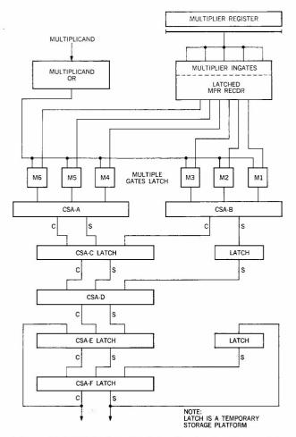
Figure 16 Multiply iterative loop showing temporary storage.
